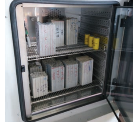
Climatic chamber with prisms for accelerated carbonation (Swiss SIA 262/1-X standard)
